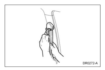
2. Feed the folded portion of the safety belt webbing through the safety belt guide (D-ring) to remove the twist from the belt webbing.
